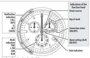
• A solar cell is placed under the dial.
