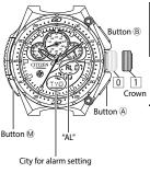
To monitor the alarm sound, press and hold button (a) for more than 2 seconds while the crown is set to position (a). You can monitor it for up to 10 seconds.
