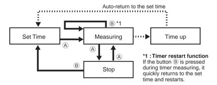
\* The mode can be changed by pressing the button (M) even during timer measuring. If it is returned to the timer mode again, the continued measuring can be displayed. If the measuring of the set time is completed, however, it returns to the set time display.
