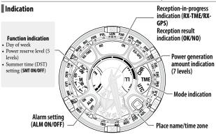
· A solar cell is placed under the dial.
