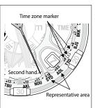
In the illustration on the left, the second hand points to 26 seconds and time zone setting is "+10.5".
