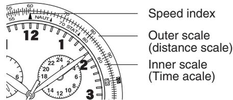
**Answer.** Align “21” on the outer scale with the SPEED INDEX (▲) on the inner scale. then, “40” on the inner scale corresponds to “14” on the outer scale. Thus, the air distance of the flight is 140 nautical miles.
