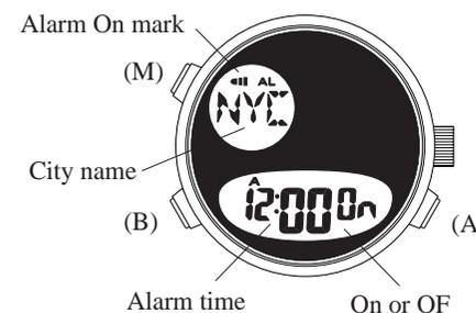
The alarm tone sounds for about 15 seconds at the same time every day once it has been set (ON). The alarm can be switched off when it is sounding by pressing any button.
