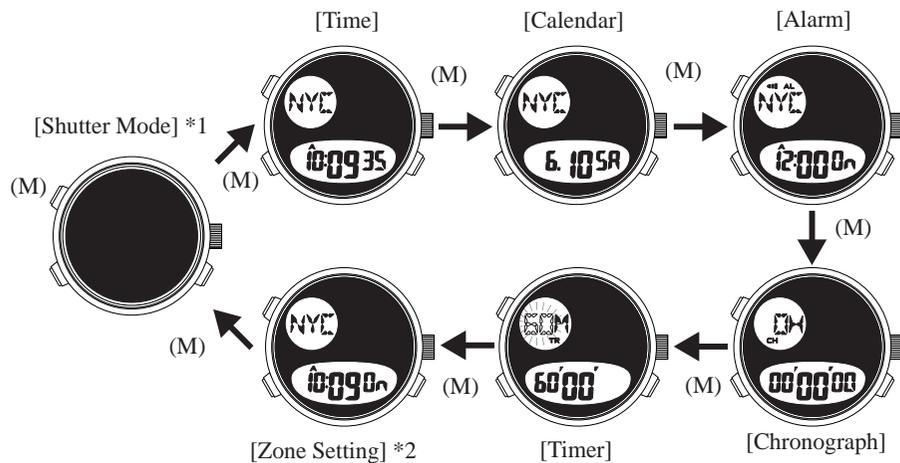
\*1: The digital display is completely concealed in the shutter mode.
