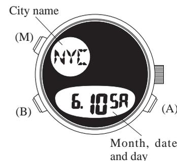
When the date is set for any of the 30 cities or UTC, the dates of other cities are automatically corrected by converting the time difference.
