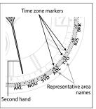
In the illustration on the left, the second hand points to 28 seconds and time zone setting is "+11.5".
