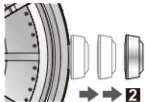
Pull out the crown just as the second hand is at the 0 second position in order to accurately align to the second.
